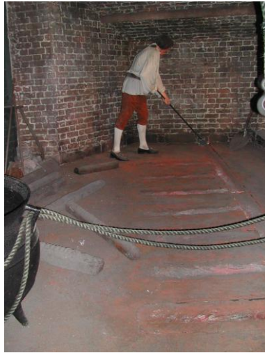
Making pig iron ingots, such as those found near the site of the Hunter's Iron Works. (Albert Z. Conner)
